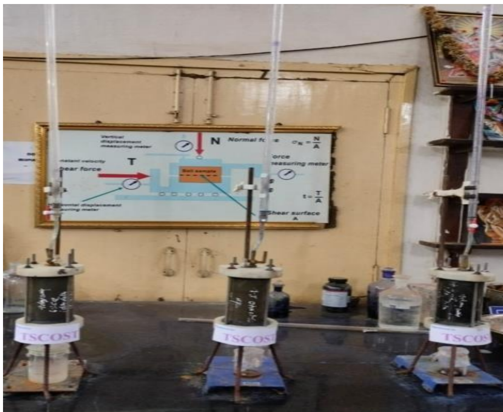
Figure 3. Leaching Apparatus for testing contaminant migration
